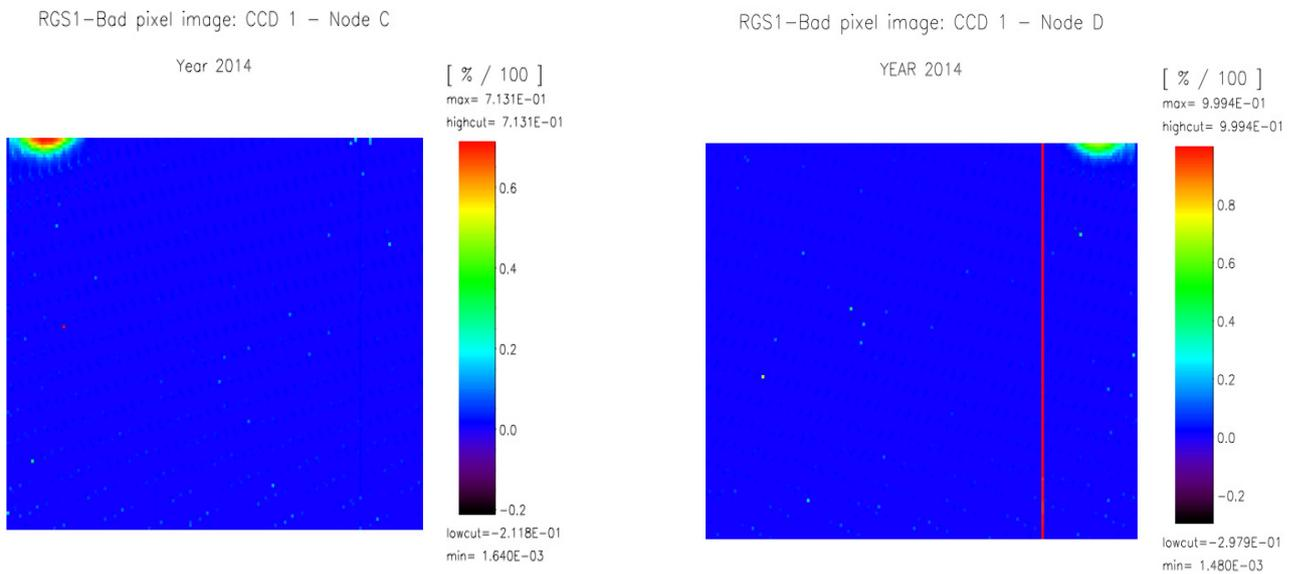
Figure 6: RGS1 - CCD1 C and D bad pixel maps showing the two "hot spots" and the only hot column found in RGS1 in the diagnostic data (column 38 on the D side) corresponding to 2014.
