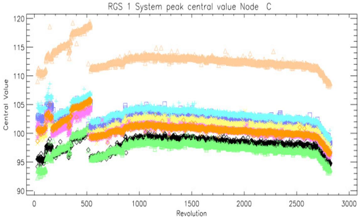
Figure 1: RGS1 - system peak evolution of node C data. Different colors represent the eight RGS1 working CCDs.
