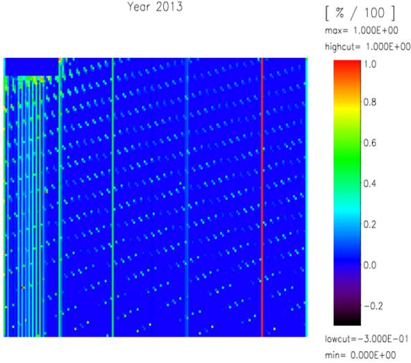
RGS1-Science Data Bad pixel image: CCD 1 - Node C
