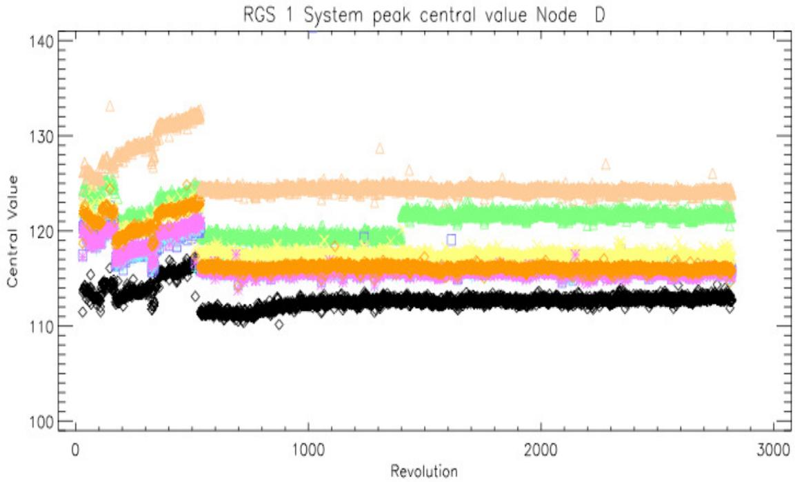
Figure 2: RGS1 - system peak evolution of node D data. Different colors represent the eight RGS1 working CCDs.
